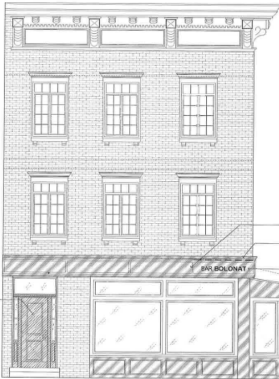
3 PROPOSED EXTERIOR ELEVATION W12 TH STREET SCALE 3/8" = 1'-0"
