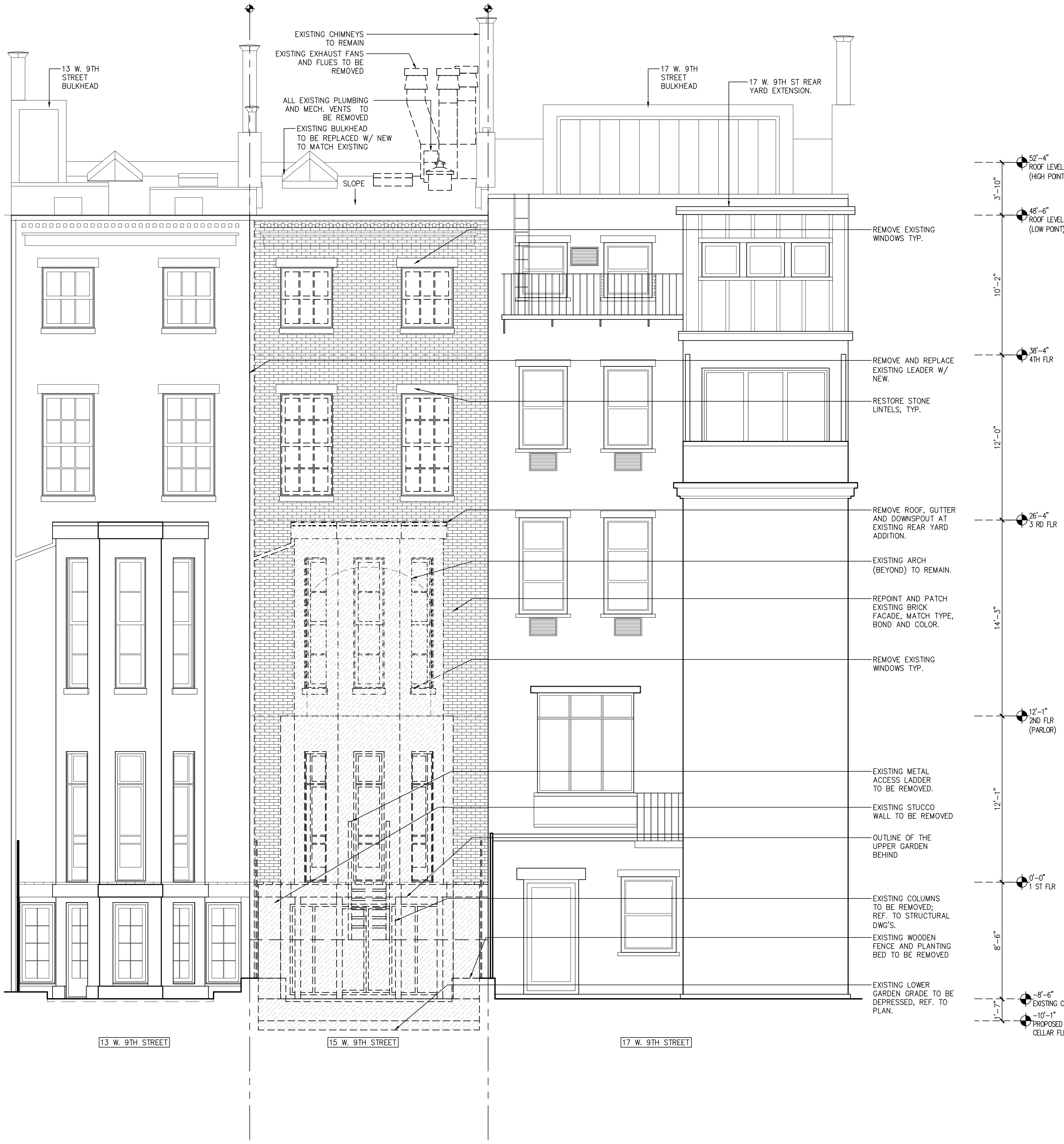
EXISTING WINDOWS AT 3RD AND 4TH FLRS TO BE REPLACED W/ NEW TO MATCH W/ EXISTING.
