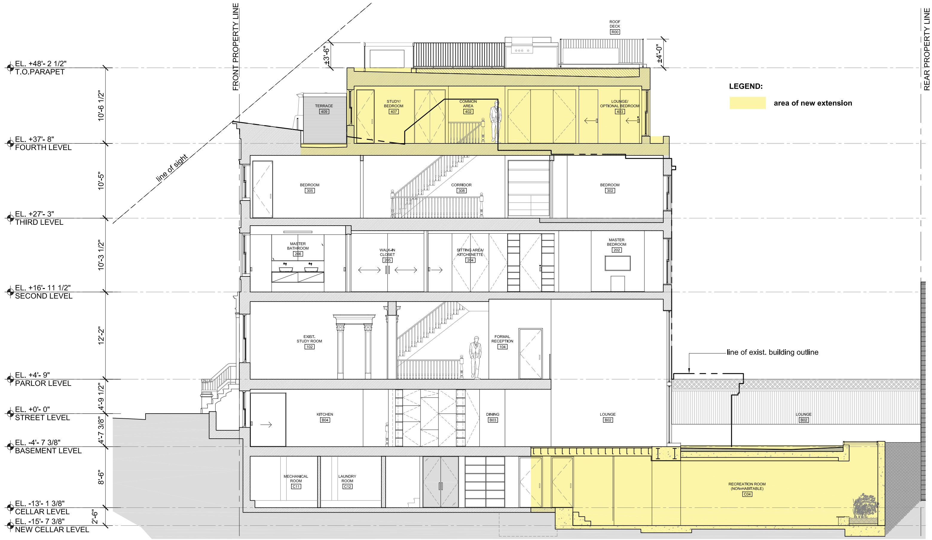
PROPOSED BUILDING SECTION: 1/8" = 1'-0"
