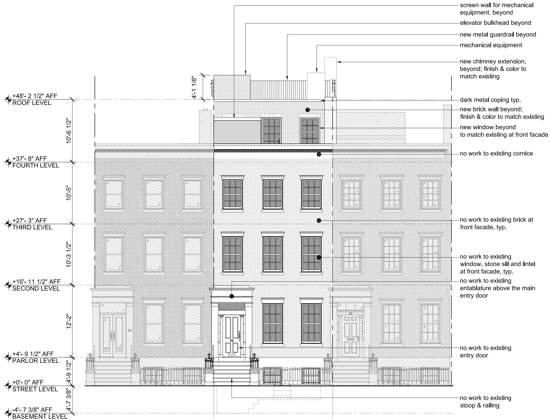
PROPOSED FRONT ELEVATION/ SCALE: 1/8" = 1'-0"
