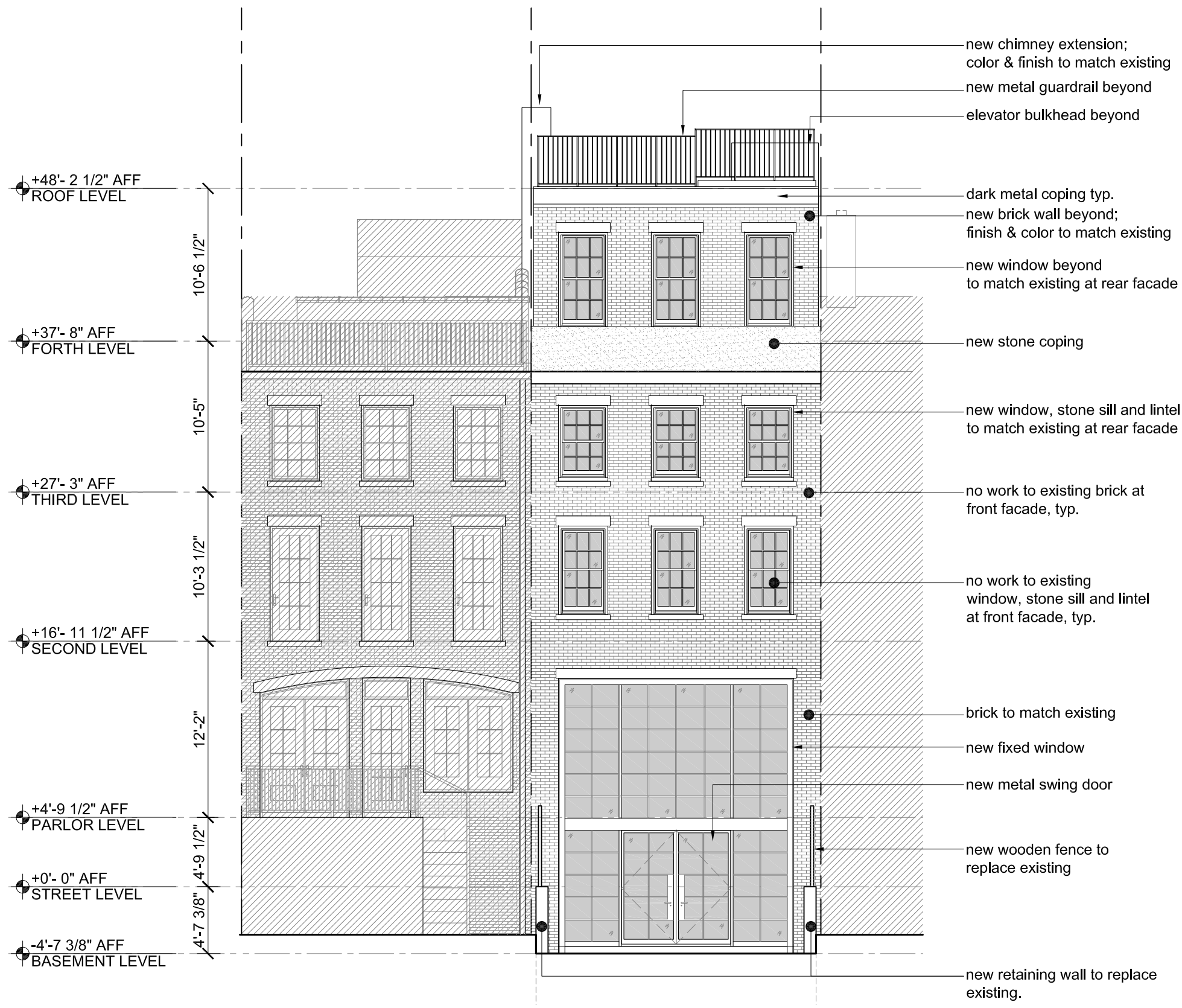
EXISTING REAR YARD ELEVATION/ SCALE: 1/8" = 1'-0"
