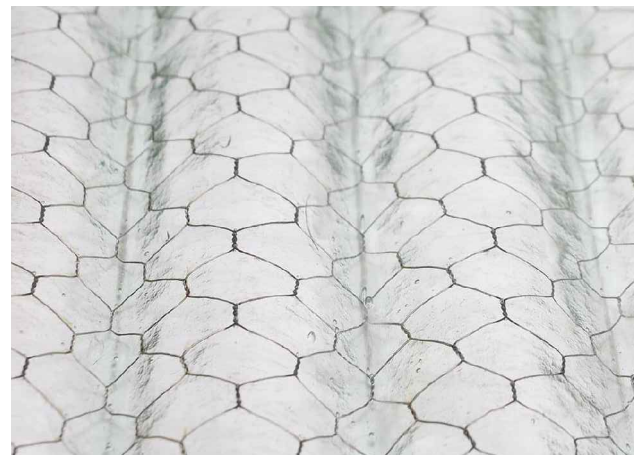
9 awning - obscure corrugated wire glass n.t.s. note: proposed awning glass to be translucent
