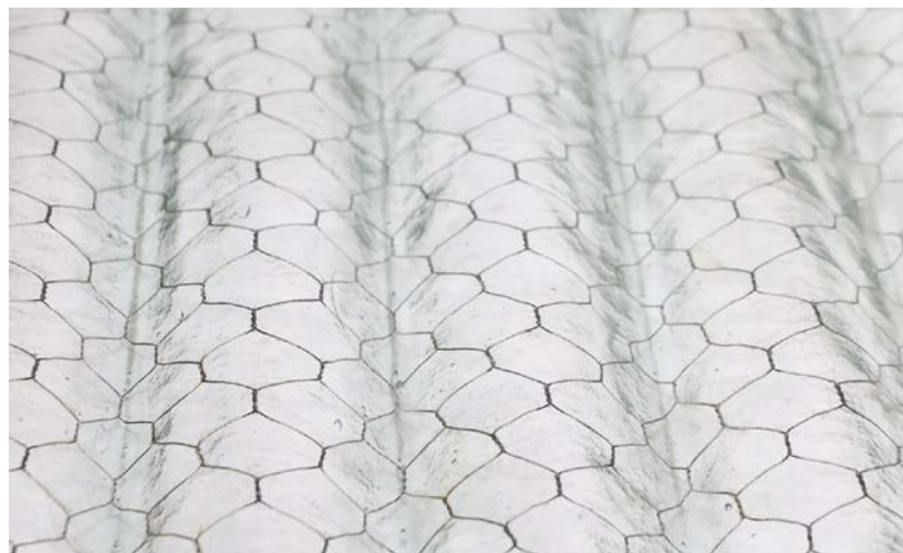
8 awning - obscure corrugated wire glass n.t.s. note: proposed awning glass will be translucent not transparent
