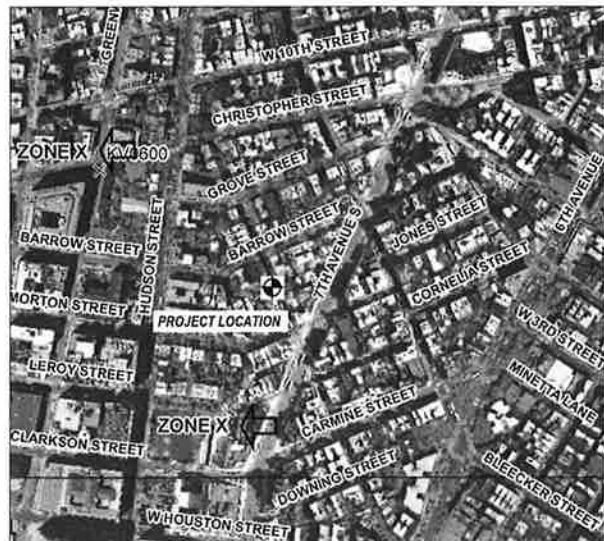
Property is located in Zone X this is not in a Special Flood Hazard Area, per revised Flood maps released September 2007.
