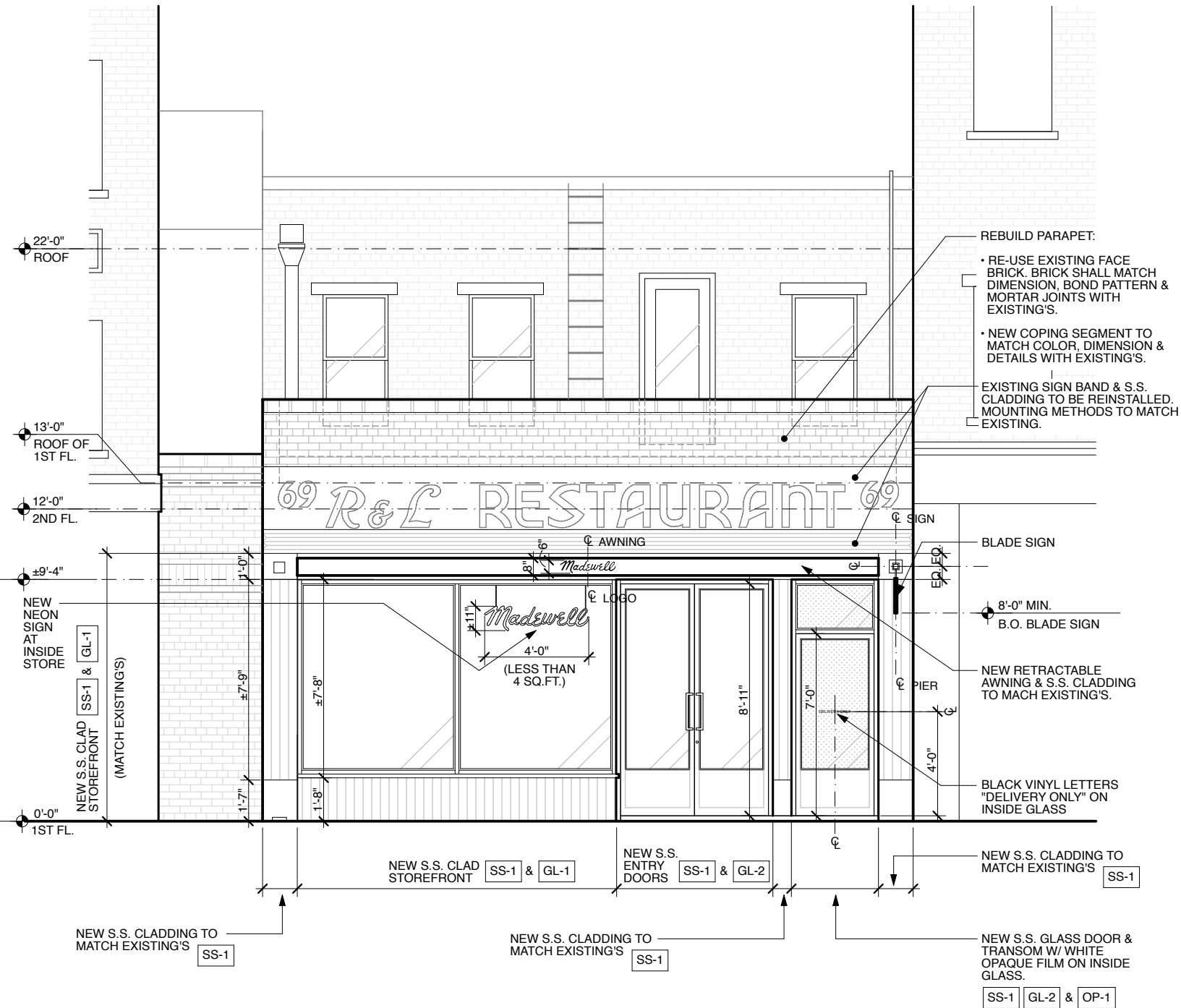
2 NEW STOREFRONT ELEVATION SCALE: 3/16" = 1'-0"
