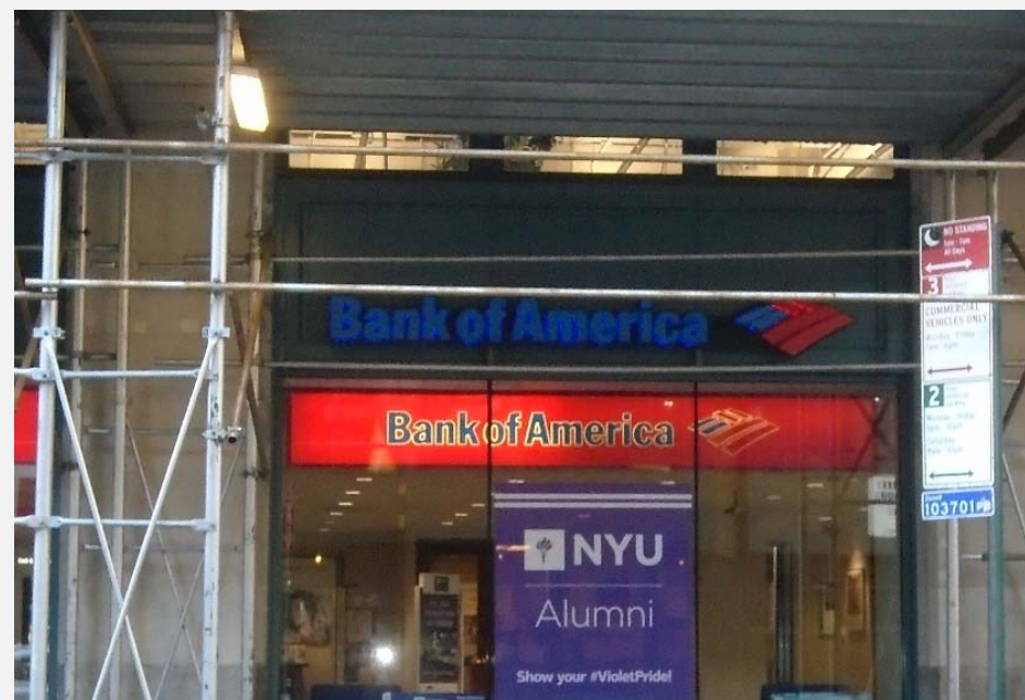
Bank of America – 770 Broadway & E 8 th Ave** • Internally Illuminated, Channel Letters
