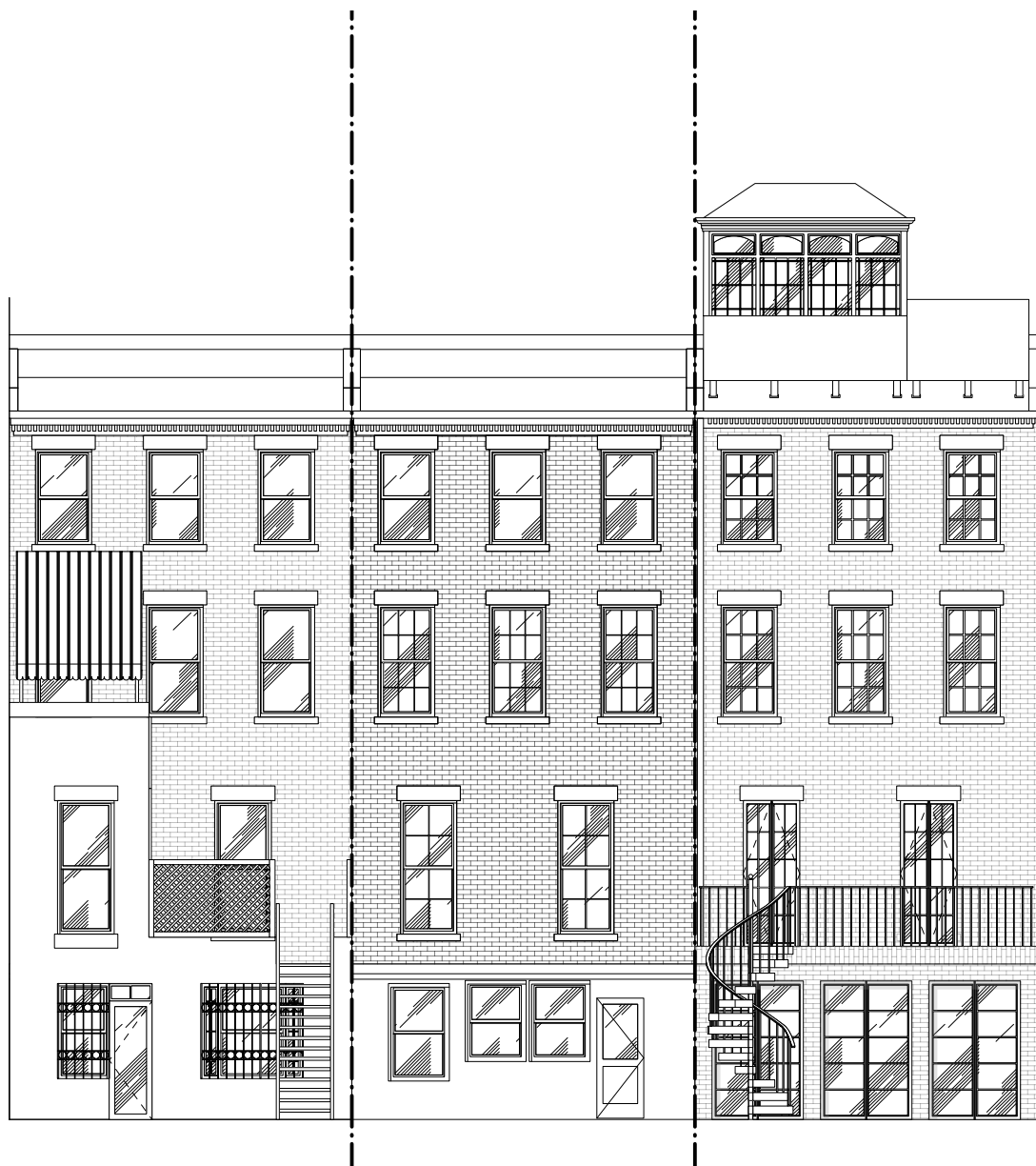
EXISTING REAR FACADE ELEVATION IN CONTEXT SCALE: 1/16" = 1'-0"
