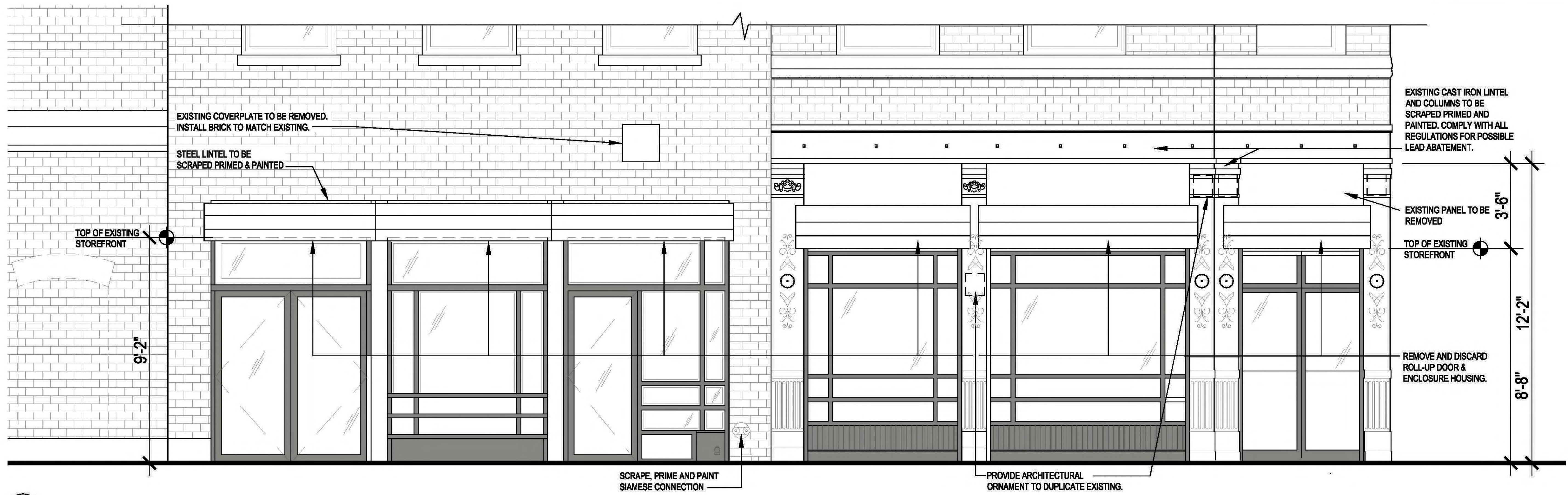
1 EXISTING STOREFRONT ELEVATION (3 & 1 BUILDING) SCALE: 1/2"=1'-0"
