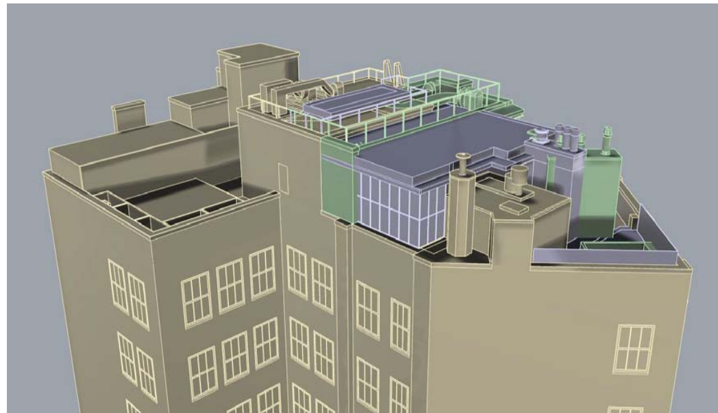
EXISTING AND REVISED PROPOSED PENTHOUSE OVERLAP WITH MULLIONS AND ROOF CUT BACK 2'-0" FROM THE SOUTH AND 8'-9" FROM THE WEST
