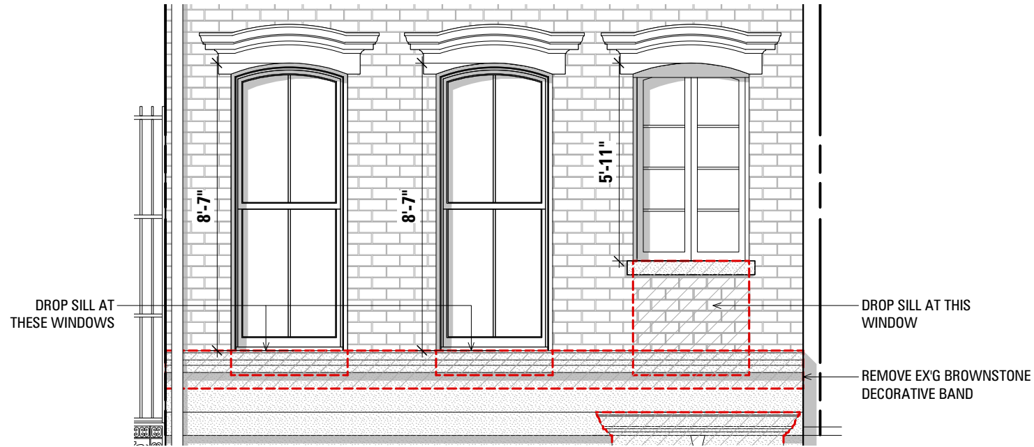
2. CLOSE-UP OF EXISTING PARLOR WINDOWS AT FRONT FACADE
