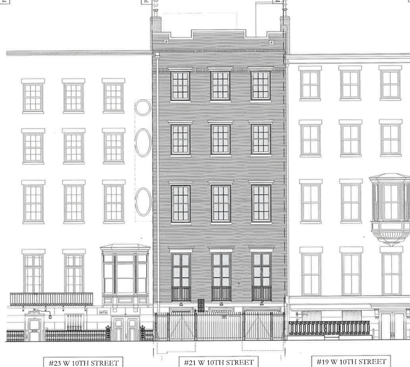
01 EXISTING FRONT ELEVATION (LEFT TO RIGHT) #23 #21 #19 WEST 10TH STREET (SOUTH FACING) LC-04 3/16" = 1'-0"
