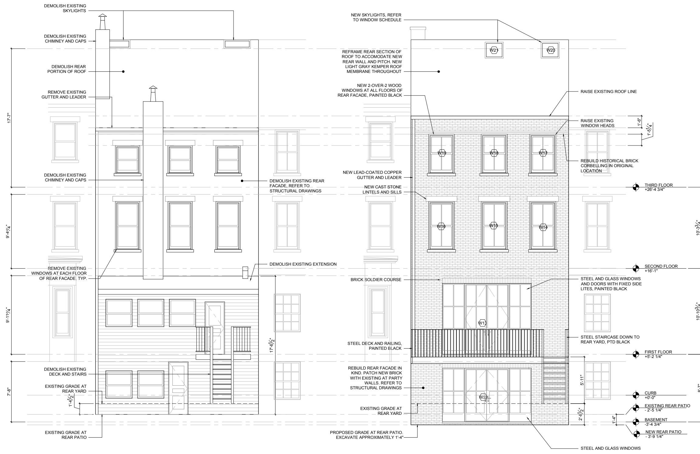
EXISTING REAR FACADE
