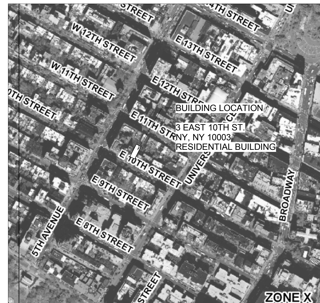
7 FLOOD MAPS 1" = 80'-0" OTHER AREAS :Areas determined to be outside the 0.2% annual chance floodplain. MAP NUMBER 3604970201F MAP REVISED SEPTEMBER 5, 2007
