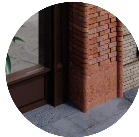
DETAIL 1: PIER BASE & STOREFRONT COLUMN
