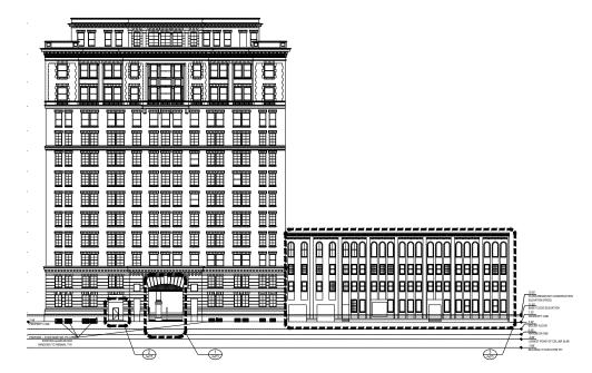
PROPOSED ELEVATION OF WEST STREET COURTYARD ENTRY - WITH ADA RAMP
