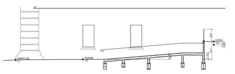
4/A304 - SECTION DETAIL 1:12 RAMP · 1½" ROUND PIPE RAIL  $1\frac{1}{2}$ " RND. RAIL MEMBER BLACK BAKED ENAMEL AL. 1-1/2" TUBE FALL PROTECTION 3'-6" 4" CONCRETE CURB W/ 2" O.D. AL. PIPE SLEEVE, W/ SEALANT GUTTER, SIM. MEIER D1/A63
