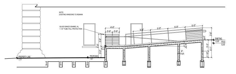
1/A501 - HANDRAIL AND FALL PROTECTION DETAIL
