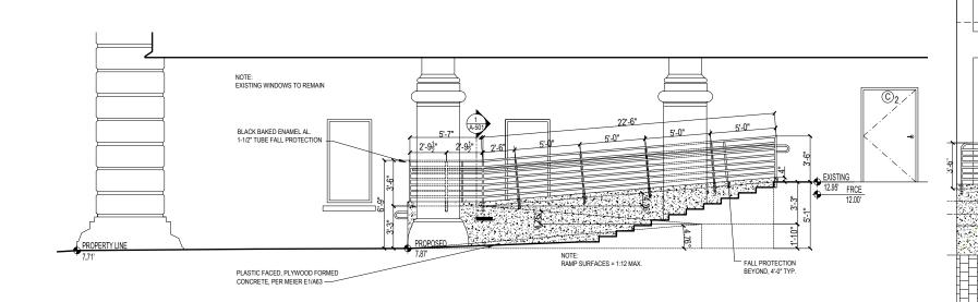
PROPOSED EAST ELEVATION - WEST STREET INNER COURTYARD ENTRY - WITH ADA RAMP
