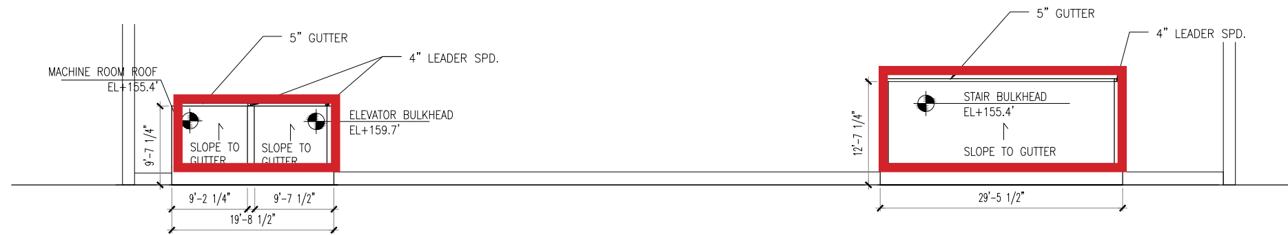
02 ROOF BULKHEAD PLAN 1/8" = 1'-0"
