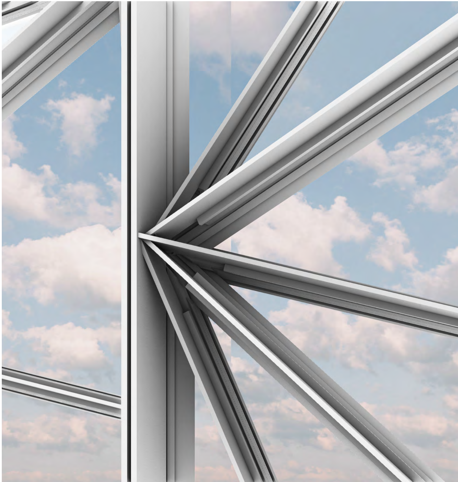
1. DETAIL VIEW OF FRAMING AT SPLIT MULLION
